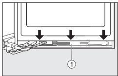
Prise open panel ① from the soft-close mechanism and ease it off carefully from above bit by bit. Take care not to damage the door seal.
